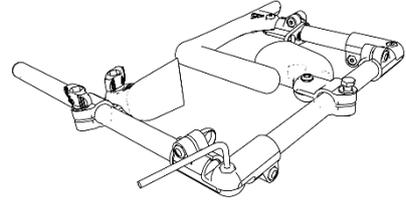
2.l- Screw all the pieces together taking care not to over tighten. You must be still able to rotate the two parts by force
