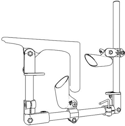
4.a- Bend all the connections at an angle of 90° so that the ProTubeVR almost forms a square
