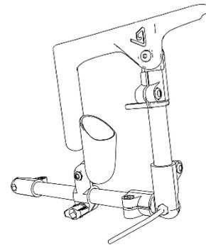
2.o- Screw all the pieces together taking care not to over tighten. You must be still able to rotate the two parts using force
