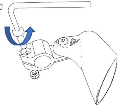
2.f- Unscrew the 18mm screw at the base of the T-notched connection.
