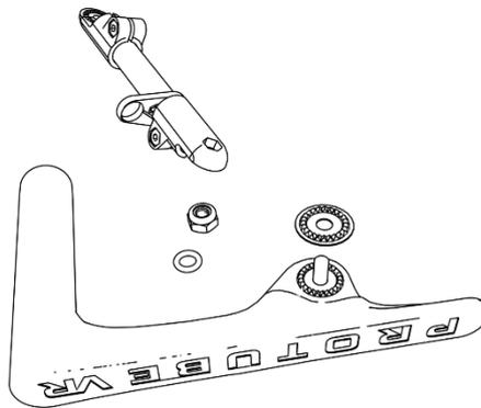
1.e- Then slide the notched washer and the previously oiled connection over the screw
