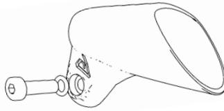
2.b- Put one O'ring on the 20mm screw, slot them both into the hole provided in the cup
