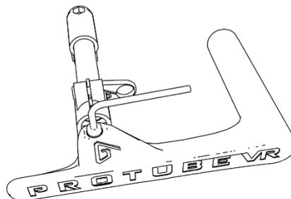
1.g- Screw all the pieces together taking care not to over tighten. You must be still able to rotate the back-end by force
