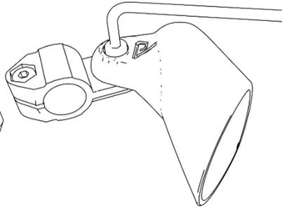
2.e- Screw all the pieces together taking care not to over tighten. You must be still able to rotate the two parts by force
