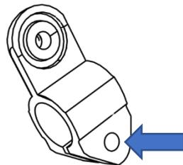
3.b- Apply a dot of oil on the base of the T-smooth connection
