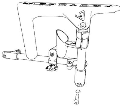
2.m- Place one O'ring on the 18mm screw (the one from 2.f), slide them both through the internal notched connection and the external connection.
