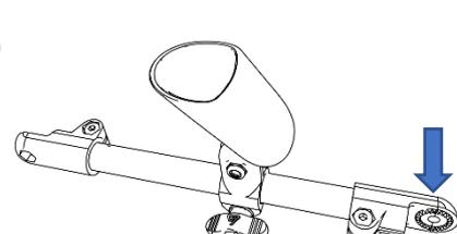
2.l- Apply some oil all around the external notches of the rear side
