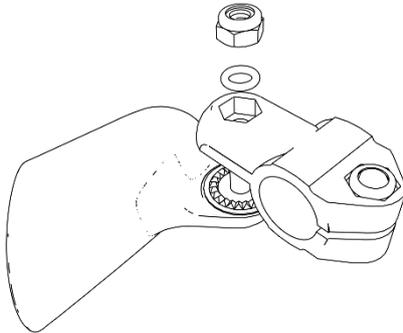
2.d- Attach the screw securing the cup and T-notched connection with one O'ring and the nut
