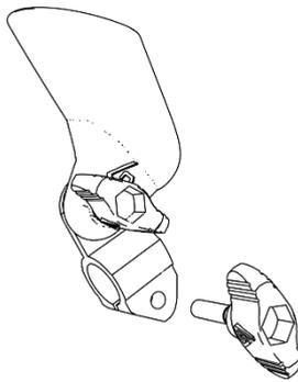
3.d- Slide the other butterfly screw through the T-smooth connection and secure it with a nut
