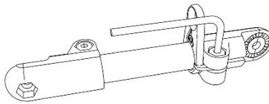
1.b- Put the two connections with internal notches on each part of the small tube and screw them with the Hex key
