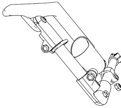
2.n- Attach the screw securing both connections with one O'ring and the nut
