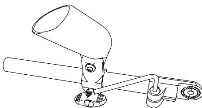
2.j- Slide the medium tube into the T-notched connection. Then place the external notches connections on both sides of the tube
