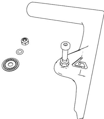
1.d- Put one O'ring on the 20mm screw, slot them both into the hole provided in the bach-end
