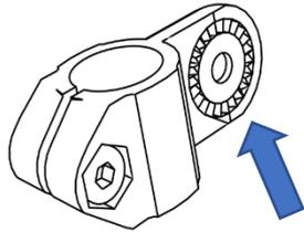
2.a- Apply some oil all around the notches on the T-notched connection
