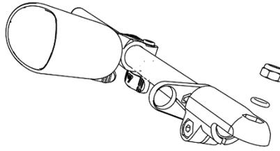
3.k- Attach the screw securing both connections with one O'ring and the nut
