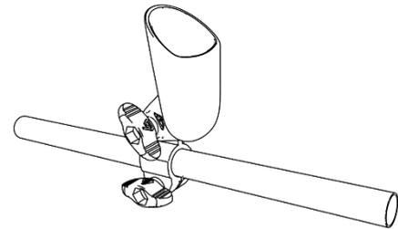
2.f- Put the previously assembled part through the long tube
