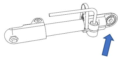
1.c- Apply some oil all around the notches on the connection which is the nearest from the ring
