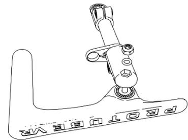
1.f- Attach the screw securing the stock and the connection with one O'ring and the nut
