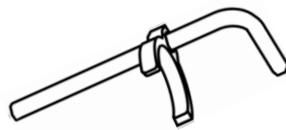
4.d- Slide the hex key through the clip so you can clip it on your ProTubeVR for later adjustments if needed
