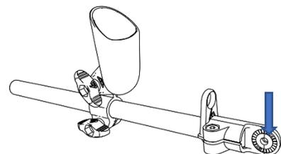
2.i- Deposit some oil around the internal notches
