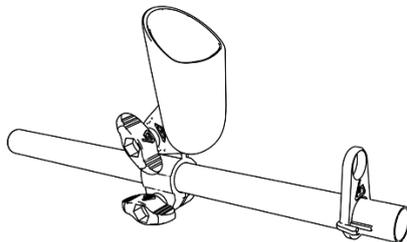
3.g- Put the wedge on the ring and slide them through the back of the tube
