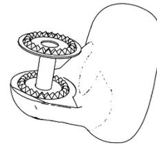
2.c- Then slide the notched washer and the previously oiled T-notched connection over the screw
