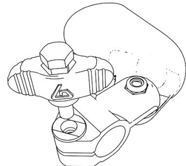
2.i- Attach the butterfly screw with the Hex screw then screw the butterfly screw with a nut on the other side
