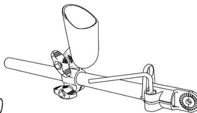
3.h- Put the connection with internal notches on the tube and screw it with the Hex key
