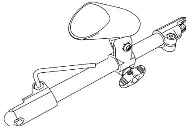
2.k- Finally screw the external notches connections on the tube
