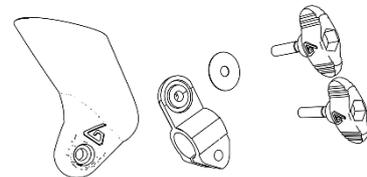
3.c- Slot one butterfly screw into the hole provided in the cup first, then into the rubber washer and finally into the T-smooth connection, secure with a nut
