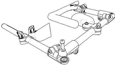
3.j- Place one O'ring on the 20mm screw, slide them both through the external notched connection and the internal connection
