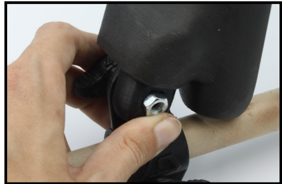
2.5. Add the magnetic support and the nut and tighten them with the butterfly, the magnetic support must be able to rotate
