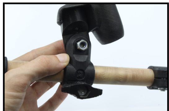
1.5. Add the nut and tighten, the magnetic support must be able to move though
